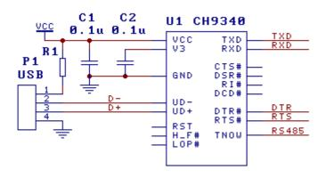
In general, the signal lines in the figure can only be connected to RXD, TXD and the public ground line. Other signal lines can be selected as needed, and can be suspended when not needed.
